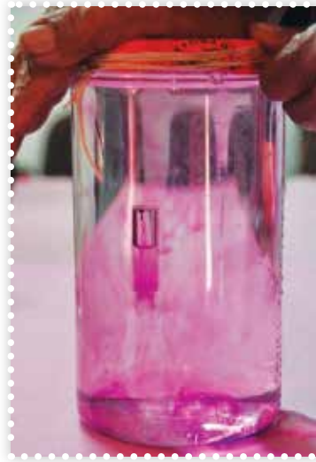
Fig. 4: On releasing the pressure, the diver coming up
